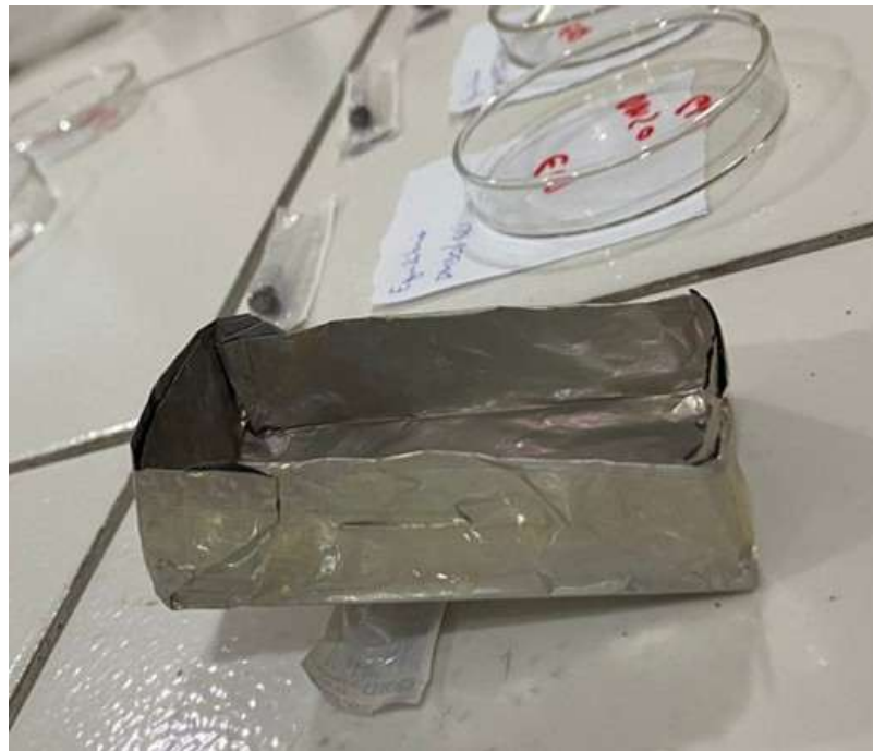
Figure 1: Metal plate for solid surface vitrification.
